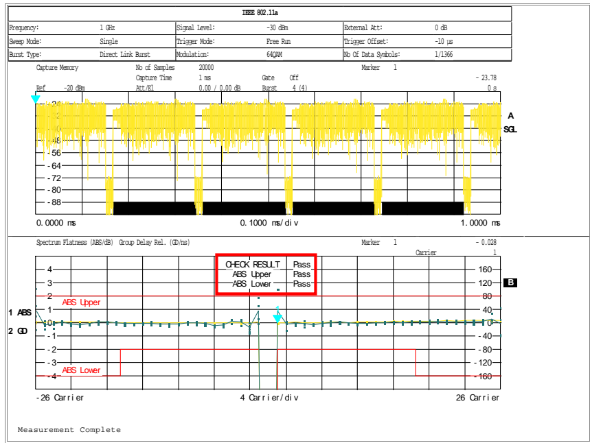
Figure 19 – Transmit spectral flatness measurement result
